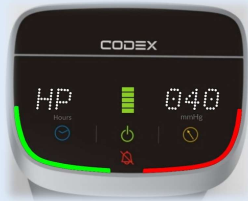
Both sleeves connected, HP Alarm for the right sleeve
