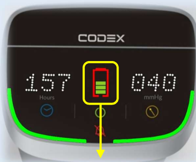
Only left sleeve connected, LP Alarm for the left sleeve
