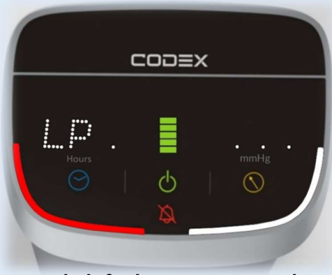
Only left sleeve connected, LP Alarm for the left sleeve
