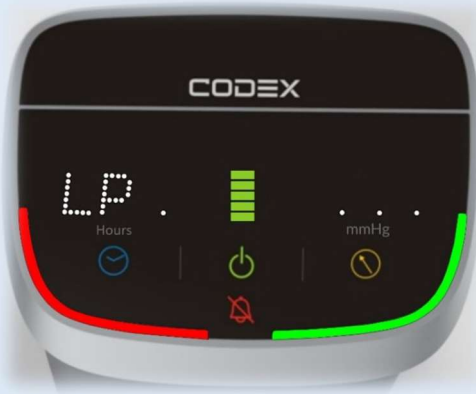
Both sleeves connected, LP Alarm for the left sleeve
