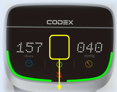
SE alarm; i.e. No sleeves connected during sleeve checking
