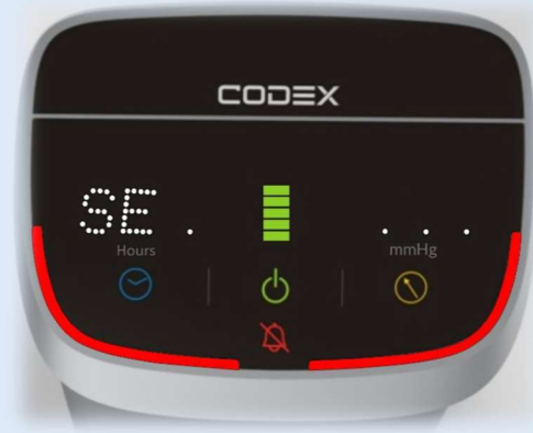
SE alarm; i.e. No sleeves connected during sleeve checking
