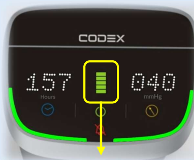
SE alarm; i.e. No sleeves connected during sleeve checking
